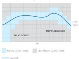
The internal 20-band equalizer in the Plantronics Voyager PRO headset automatically adjusts to background noise to maintain a natural-sounding voice quality. Headsets without Plantronics AudiolQ<sup>2</sup> technology tend to sound either too tinny or too muffled.
